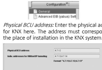
Figure 8: Config Tool – address for KNX
